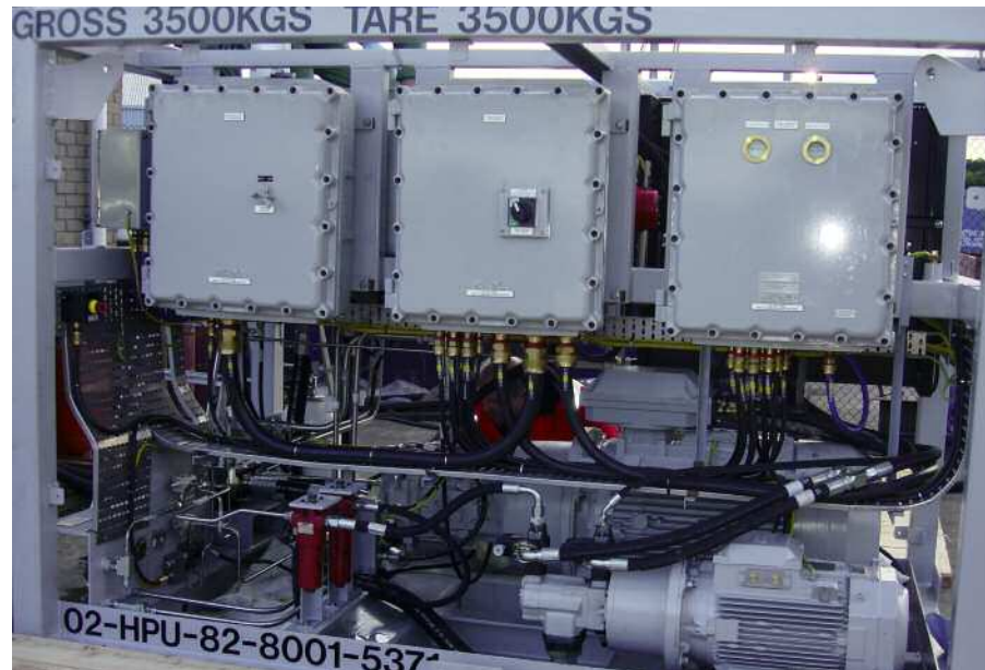
Electric driven Hydraulic power unit designed for gas turbine project
