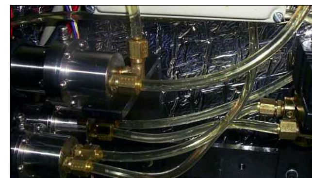
Delphi's automotive division in Spain uses custom-built flowmeters to test a range of petrol and diesel fuel injectors manufactured by the company
